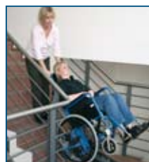
Klittervorgang starten. begin to ascend or descend stairs .
