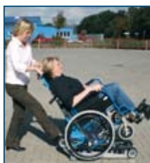
kippen und an die Treppe fahren... recline the passenger and move him to the stairway...
