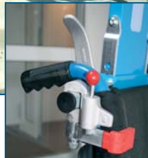
sichere Befestigung des Rollstuhls am Treppenkuli safely attaching the wheelchair with a clamp on each side...
